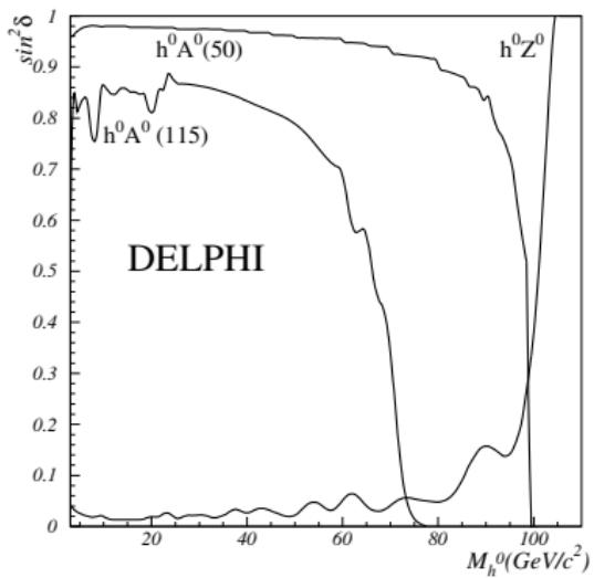
DELPHI  $hA + Zh$  combination excludes most  $(m_h, m_A)$  accessible at LEP-II energies for exactly fermiophobic models [hep-ex/0406012].
